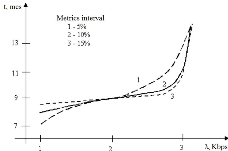
Fig. 6. Dependence of information delivery time on traffic in case of communication channel failure for a given interval of balancing group metrics
