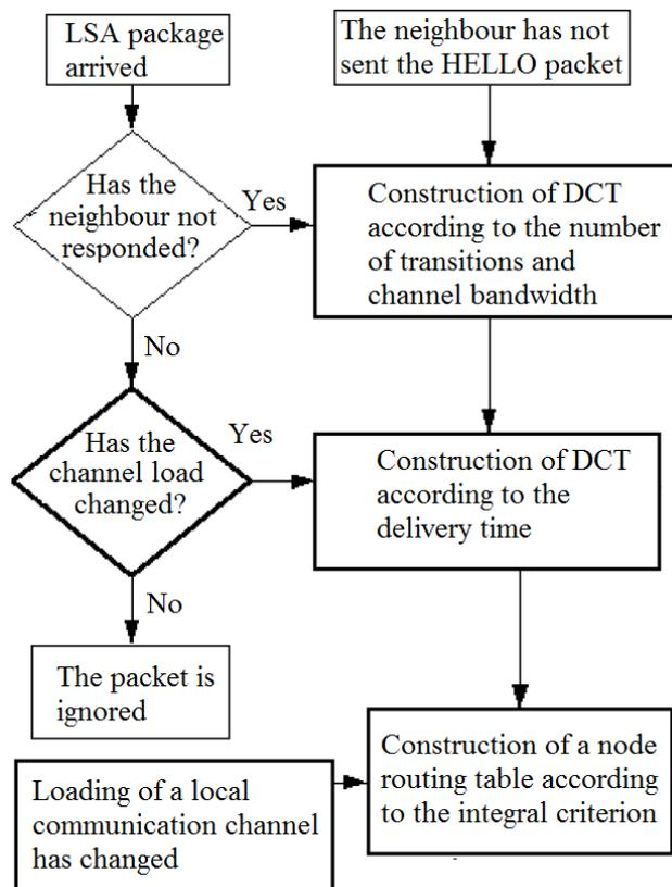
Fig. 3. Algorithm for packet processing by the switch subsystem
