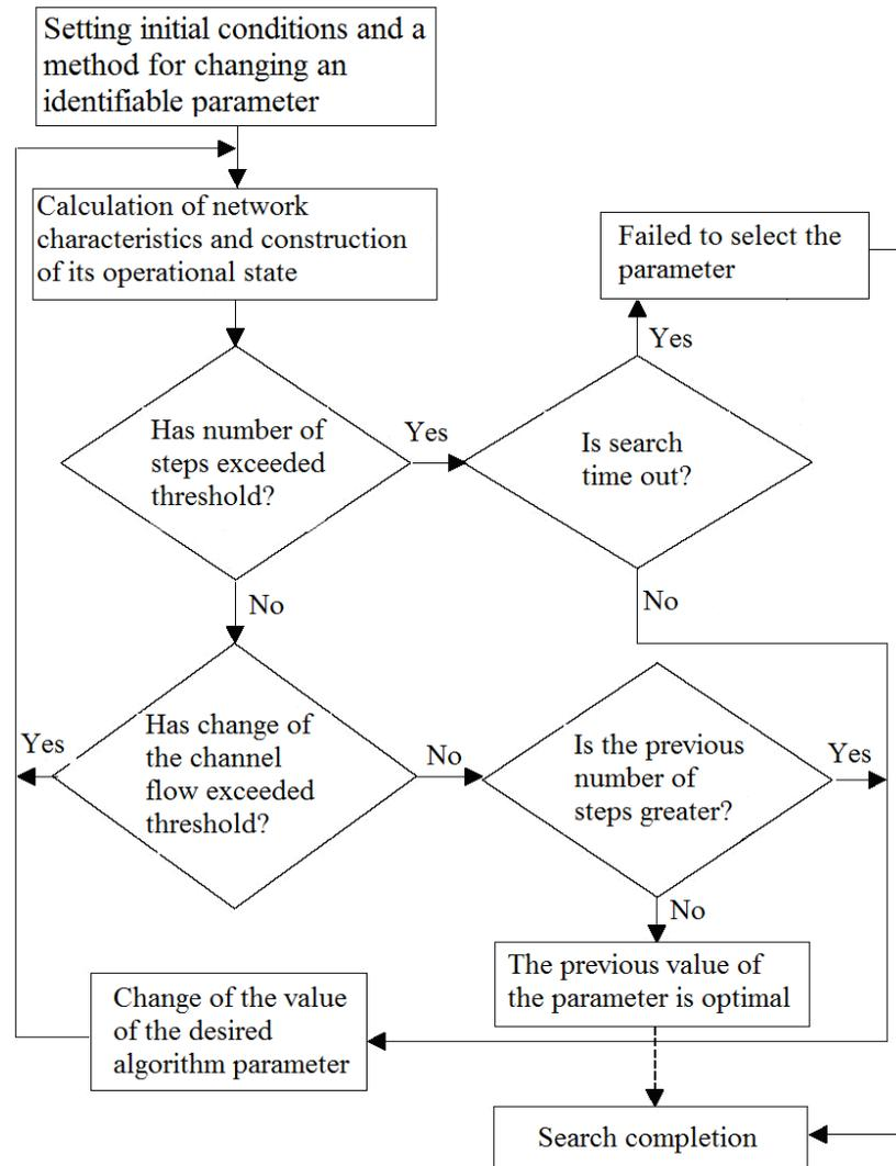
Fig. 1. Algorithm for identifying the parameters of the routing process model
