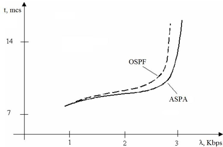
Fig. 5. Dependence of delivery time on inter-node traffic
