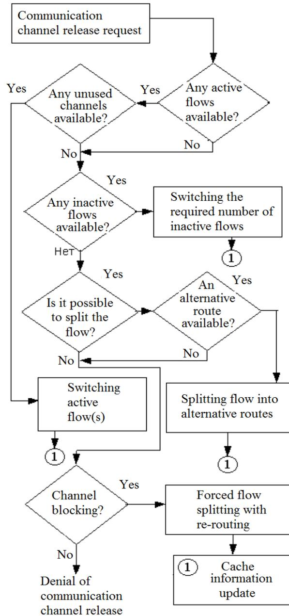
Fig. 4. Flow switching algorithm
