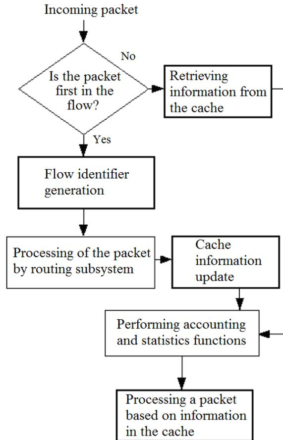
Fig. 2. Algorithm for constructing route tables
