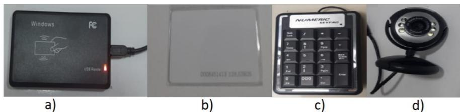
Fig. 2. Hardware components – a) RFID Reader; b) RFID Chips; c) Numeric pad; d) Camera
