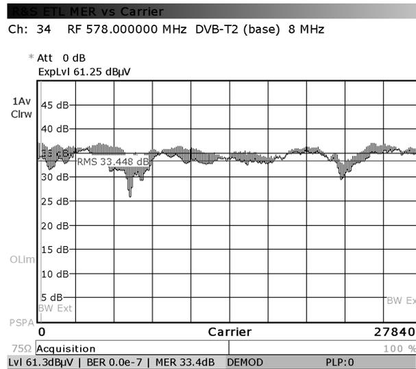
Fig. 7. Merograma with transmitted power level at 80%.
