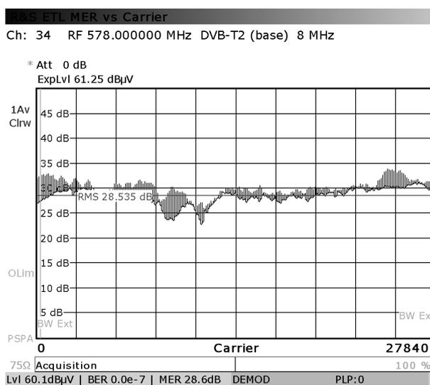
Fig. 9. Merograma with transmitted power level at 60%.
