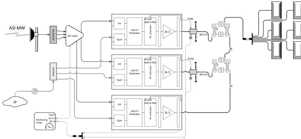
Fig. 1. Three channel DVB-T2 transmitter chain.
