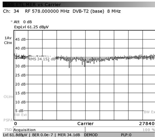
Fig. 6. Merograma with transmitted power level at 90%.
