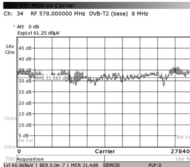
Fig. 8. Merograma with transmitted power level at 70%.
