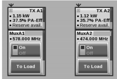
Fig. 5. Monitoring and relative efficiency for two active transmitters.
