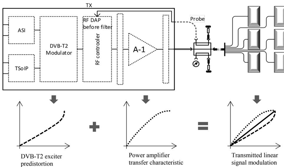
Fig. 2. Logical concept of predistortion behaviour.
