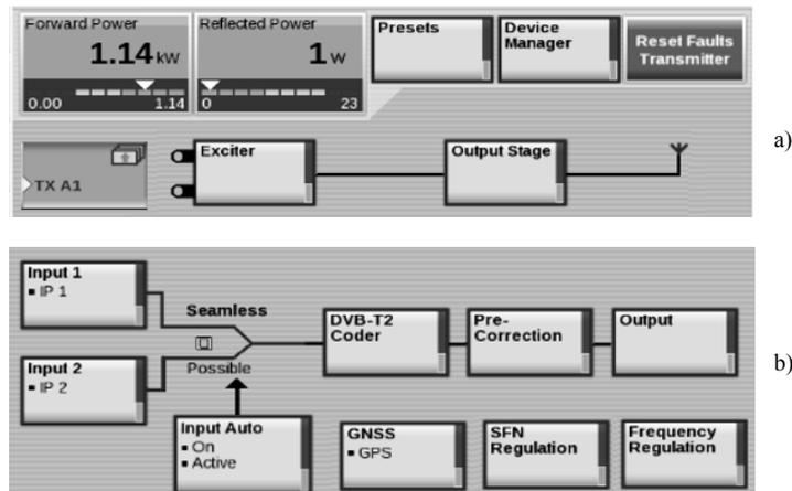
Fig. 3. Transmitter configuration: a) Exciter -> PA; b) Exciter configuration.
