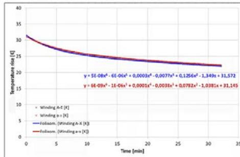
Temperature-rise test (400A – 5 min)
