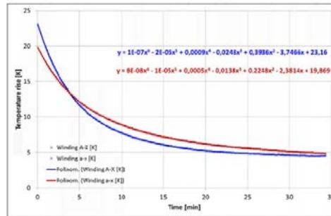
Temperature-rise test (700A – 1 min)
