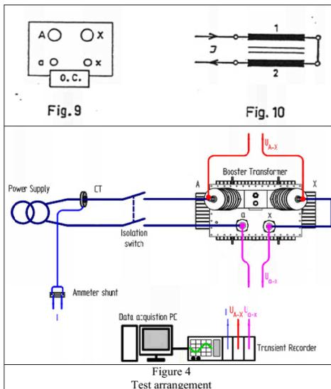
Fig. 2. Routine Test and Temperature-rise Test arrangement
