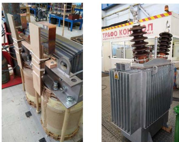
*Fig. 5. Manufactured Booster Transformer (200 Amps) subject to research*
