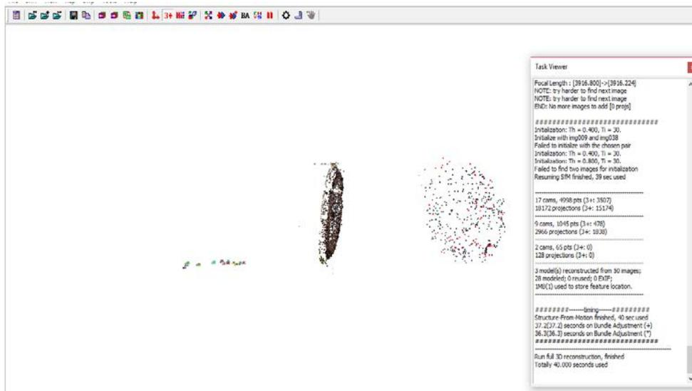
Fig. 1. A point cloud of a cylindrical object obtained in VisualSFM.
