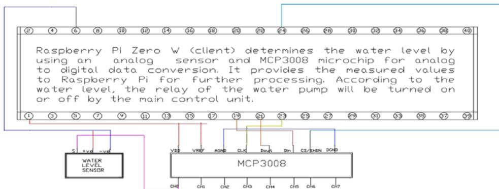
Fig. 2. Client connection with the Water level and the A/D converter
