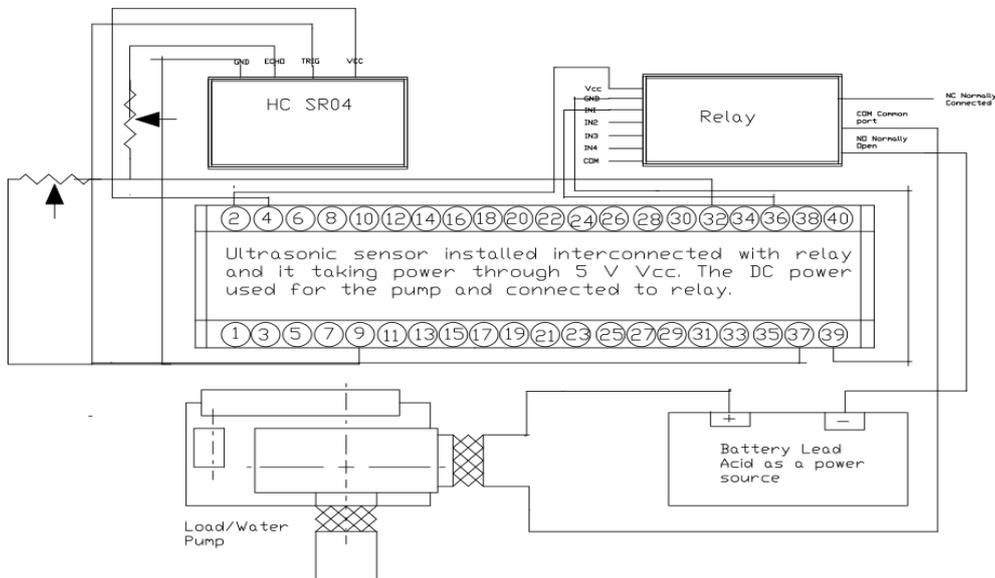
Fig. 3. Automation of water pump and relay
