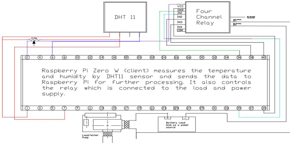
Fig. 1. Circuit Diagram of the DHT 11 sensor with relay
