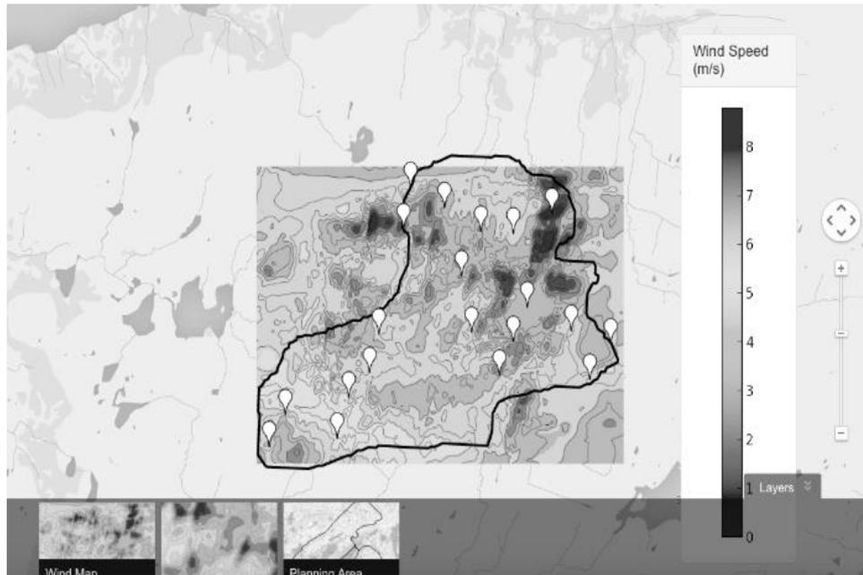
Fig. 9. Computed windfarm with a 20 turbine layout
