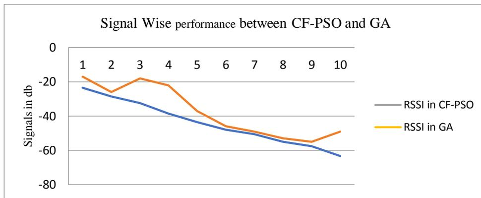
Fig. 6. Signal Wise performance between CF-PSO and GA
