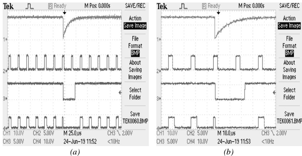
Fig. 4. Oscillograms of experiment: (a) time base 25 $\mu$ S/div; (b) time base 10 $\mu$ S/div, CH1 – IC U2 – pin2; CH2 – pulses from controller; CH3 – protection to controller; CH4 – pulses to drivers.
