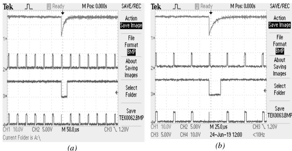
Fig. 5. Oscillograms of experiment: (a) time base  $50\mu\text{s}/\text{div}$ ; (b) time base  $25\mu\text{s}/\text{div}$ , CH1 – IC U2 – pin2; CH2 – pulses from controller; CH3 – protection to controller; CH4 – pulses to drivers.
