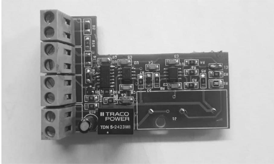
Fig. 3. Appearance of the developed and tested protection circuit.
