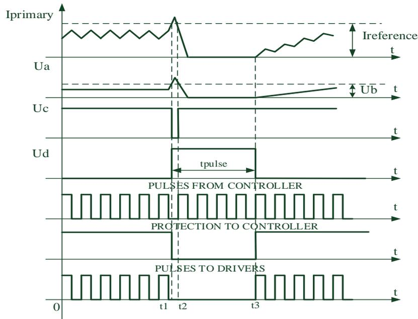
Fig. 2. Time diagrams, illustrating the operation
