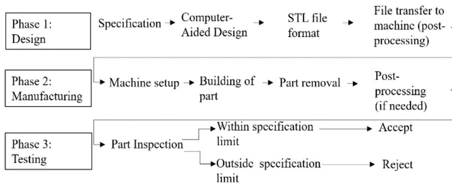
Fig. 1. Phases of Additive Manufacturing
