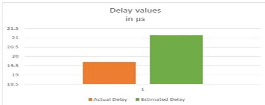
Fig. 7. Average actual and estimated end-to-end delay time in scenario 1
