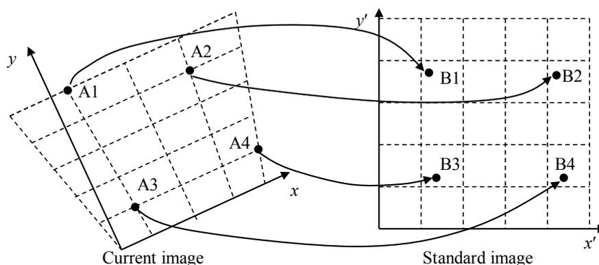
Fig. 1. Principle of geometric transformations
