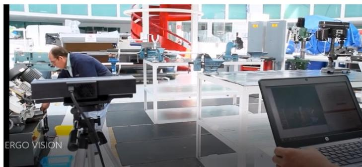
Fig. 4. Placement of the equipment for the continuous study of worker movements
