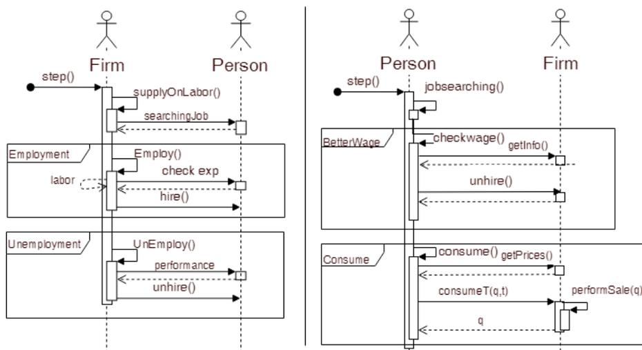
Fig. 4. Person-Firm Sequence Diagram
