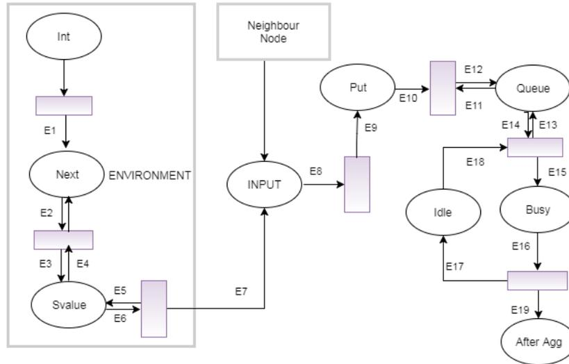
Figure 5. CPN model of the cluster head node
