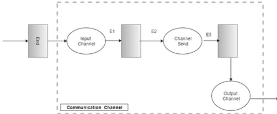
Figure 3. CPN model of the communication channel
