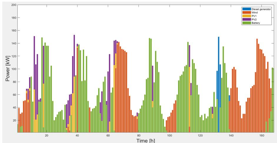
Fig. 7 Optimal scheduling of the units installed in the analysed stand-alone system
