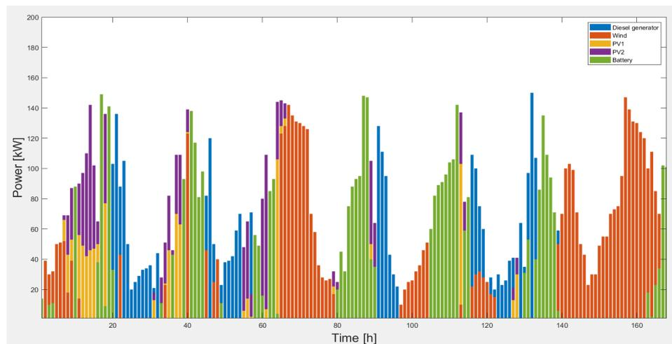
Fig. 6 Optimal scheduling of hybrid system with a 300 kWh battery capacity
