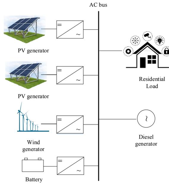
Fig. 3. Hybrid stand-alone system test example
