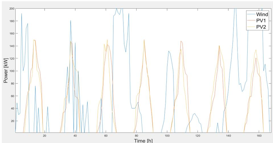
Fig. 5. Hourly power generation from the wind and PV generators
