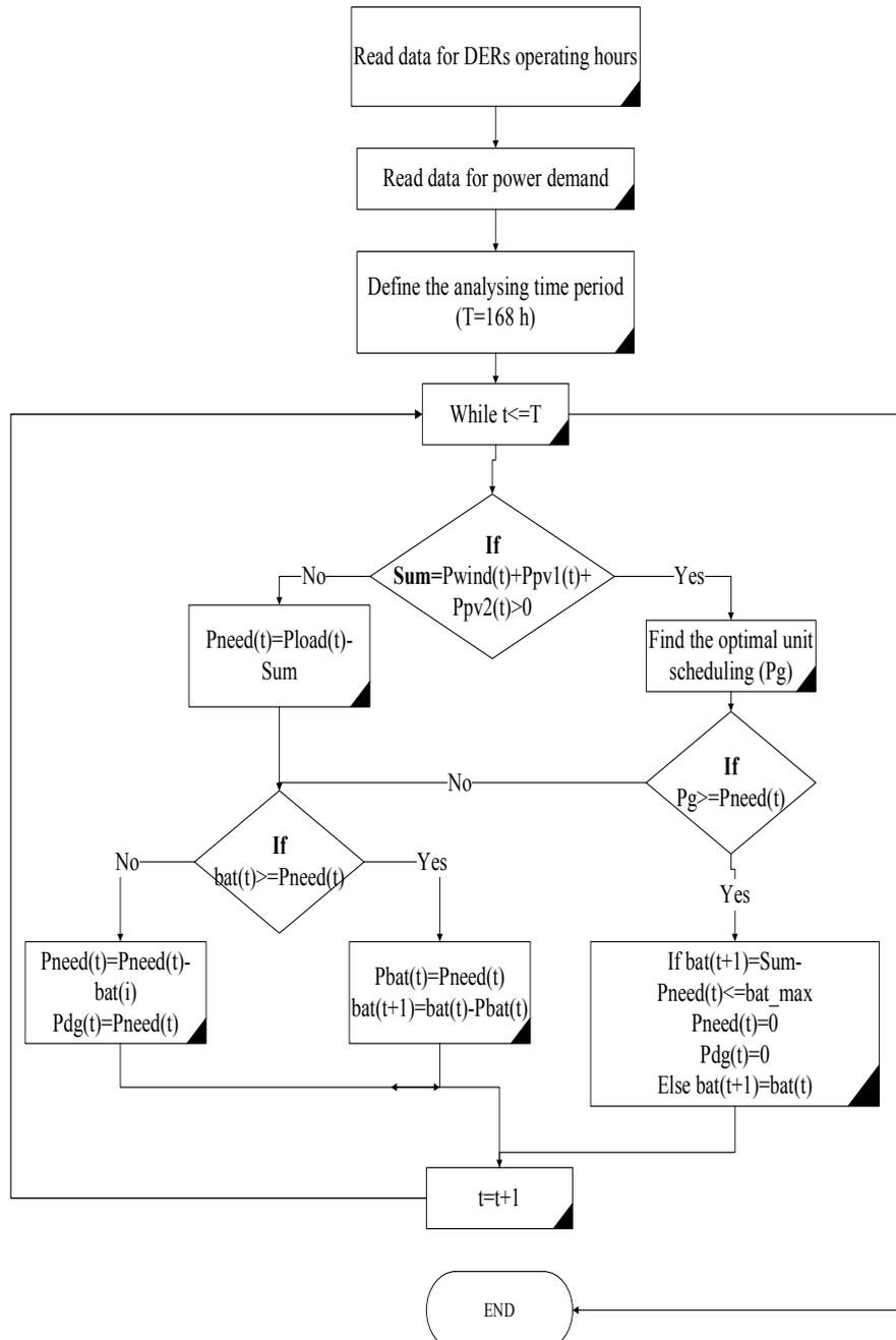
Fig. 2. Flowchart of the proposed algorithm for solving the unit commitment problem in a hybrid stand-alone system
