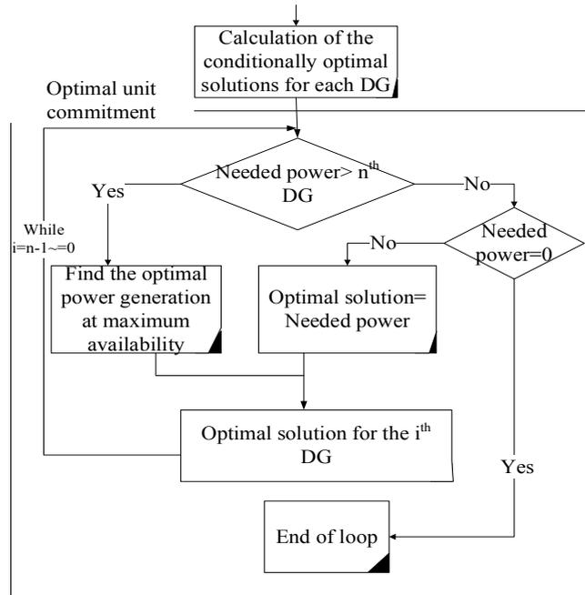
Fig. 1. Flowchart of the dynamic programming-based algorithm for finding the optimal unit commitment
