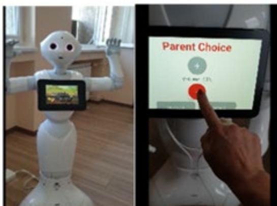
Fig. 1. Softbank's robot Pepper: a) dimensions and gestures; b) Pepper tablet
