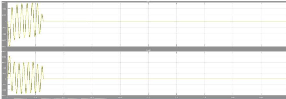
Figure 10. Stator and rotor current after activating the protection system
