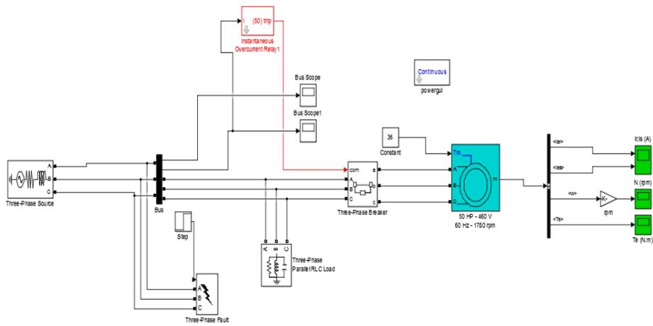
Figure 13. Second model over current fault and protection system
