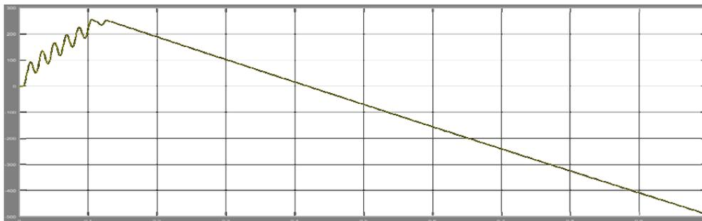
Figure 16. Rotor speed after activating the protection system
