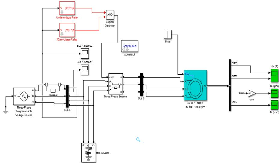
Figure 2. First model under voltage, loss of one phase and asymmetric power supply protection
