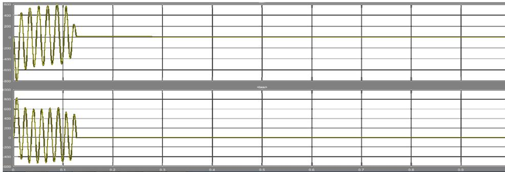
Figure 15. Stator and rotor current after activating the protection system
