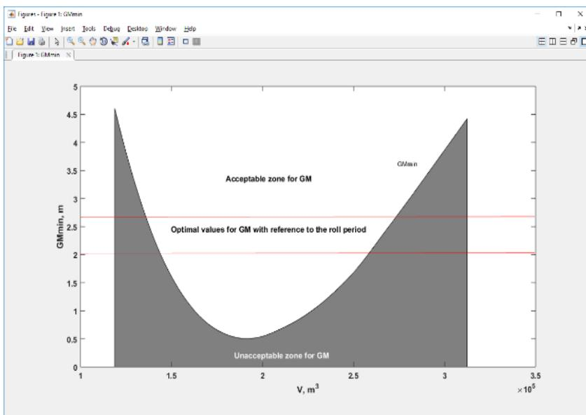
Fig. 7. Limited curve for minimum acceptable  $\overline{GM}$
