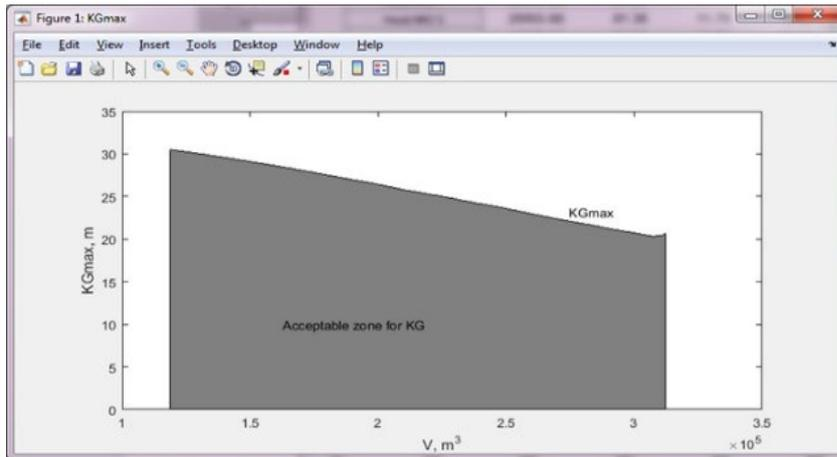
Fig. 6. Limited curve for maximal acceptable  $\overline{KG}$
