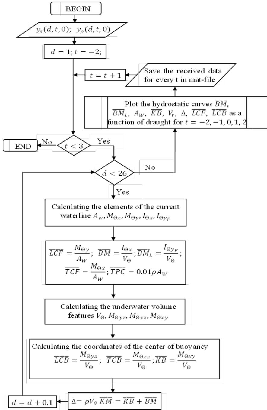
Fig. 5. Flow chart of the predefined process "Calculating hydrostatic curves at  $\theta = 0^0$ "
