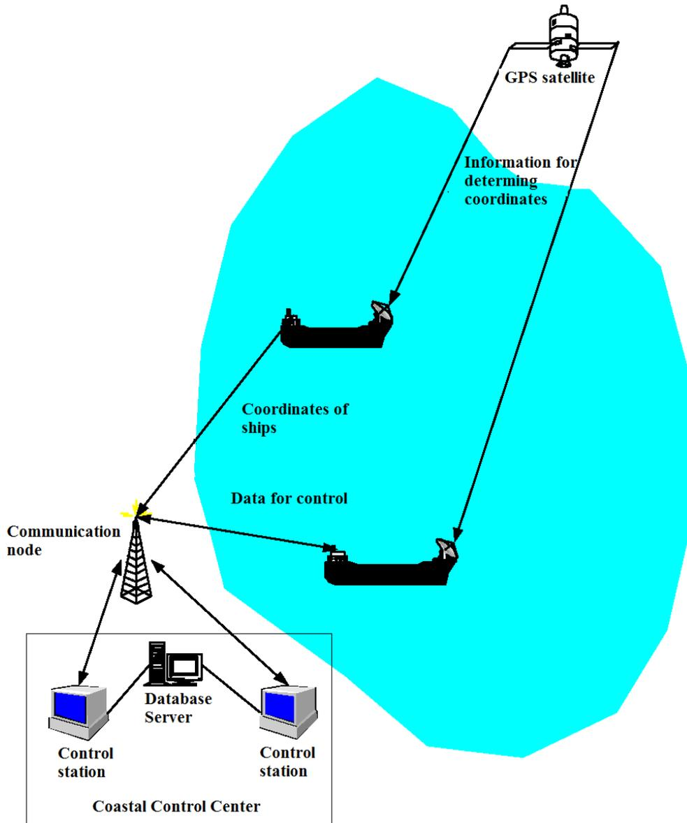
*Fig. 2. Structure of the ship traffic remote control system*
