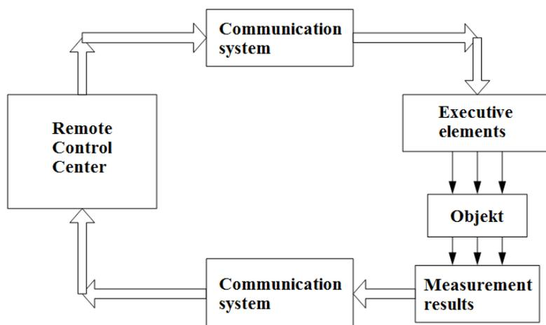
*Fig. 1. The general block diagram of the remote control system of an unmanned vessel*
