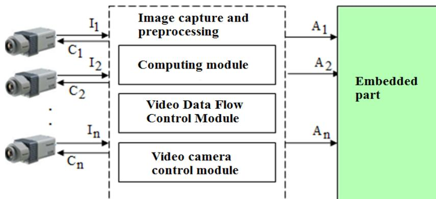
Figure 2. Block diagram of the structural components of the image capture and preprocessing module
