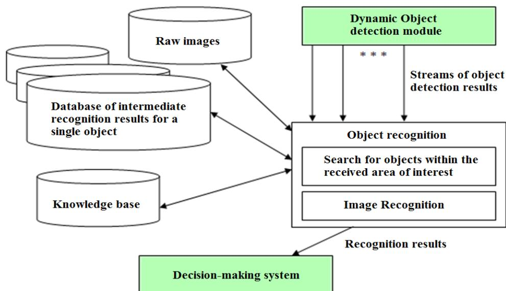
Figure 3. Data flow diagram of the pattern recognition module
