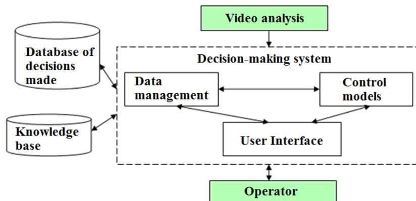
Figure 6. Block diagram of the decision support system
