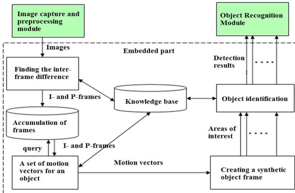
Figure 4. A model for processing a single stream of video data
