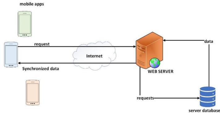
Figure 3. Synchronization module architecture
