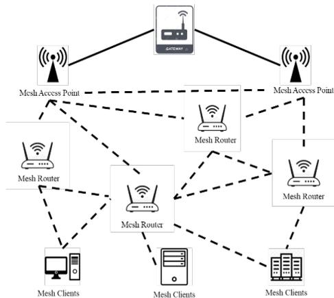
Figure 1. Topology for WirelessHART Mesh Network [12]
