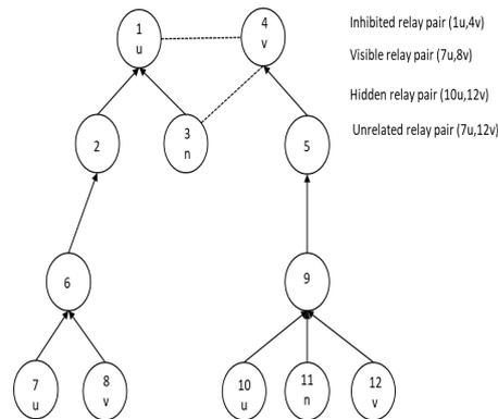
Figure 2. Device pair classification for IEEE 802.11s wireless mesh network.
