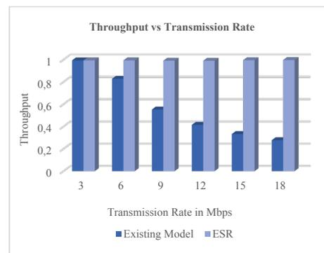
Figure 4. Throughput vs Transmission Rate.
