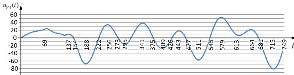
Fig. 5. The response of the object to the test signal in the form of the sum of the third, fourth and seventh harmonics
